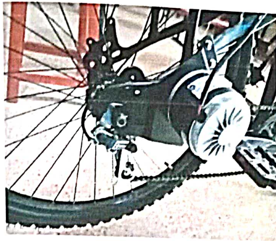
Fig 4.1: View of PMDC motor fixed to the rear wheel of the bicycle
